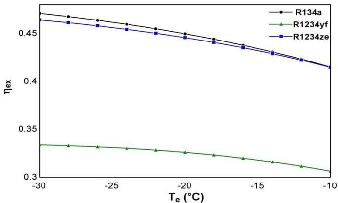
Figure 6: Variation in exergy efficiency with evaporator1 temperature
