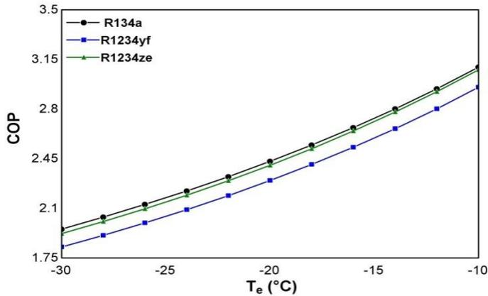
Figure 5: Variation in COP with evaporator1 temperature
